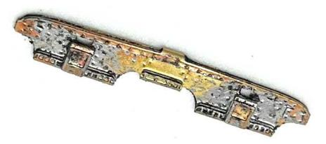
Glue the skirts on the frame. If you align on the top, the holes for the wheel axles should be open to received the wheels. Insert the wheels and see if they run freely.
