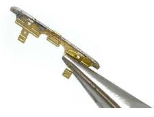
Put solder or super glue on the parts that you've just folded, so all parts fall on top of each other. This includes the "harmonica", which now can be closed completely. Make sure the alignment is correct. Check the back so that the holes are aligned.
