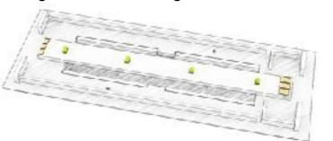
Take the Train-O-Matic LED light strip (B-16) and cut it to size, as shown on the picture. Tape it with double sided tape to the roof, the part where it is cut to the rear of the train.
