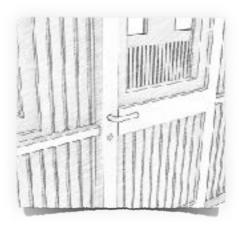
Fit handle bar (A-3C). Make sure if fits straight by cutting the bottom pin short. The end of the hole is ending against the bottom plate of the model.
